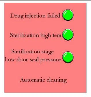
6. High temperature alarm display. It indicates that the temperature of the inner tank or water tank is too high. The device will automatically end the work. If the medicine has been added, it will automatically enter the residual discharge program. First, check whether there is a problem with the set parameters. Second, check whether there is a problem with the water tank and water source. Third, check whether the heating relay is burned out.
