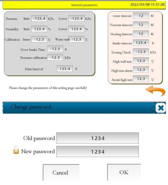
6. Manual test interface. This interface is generally only used for testing or in emergency situations. It is used when the device has stopped automatic operation.
